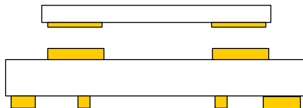
Figure 19. Correct PCB Top Metal Pattern Under Package
